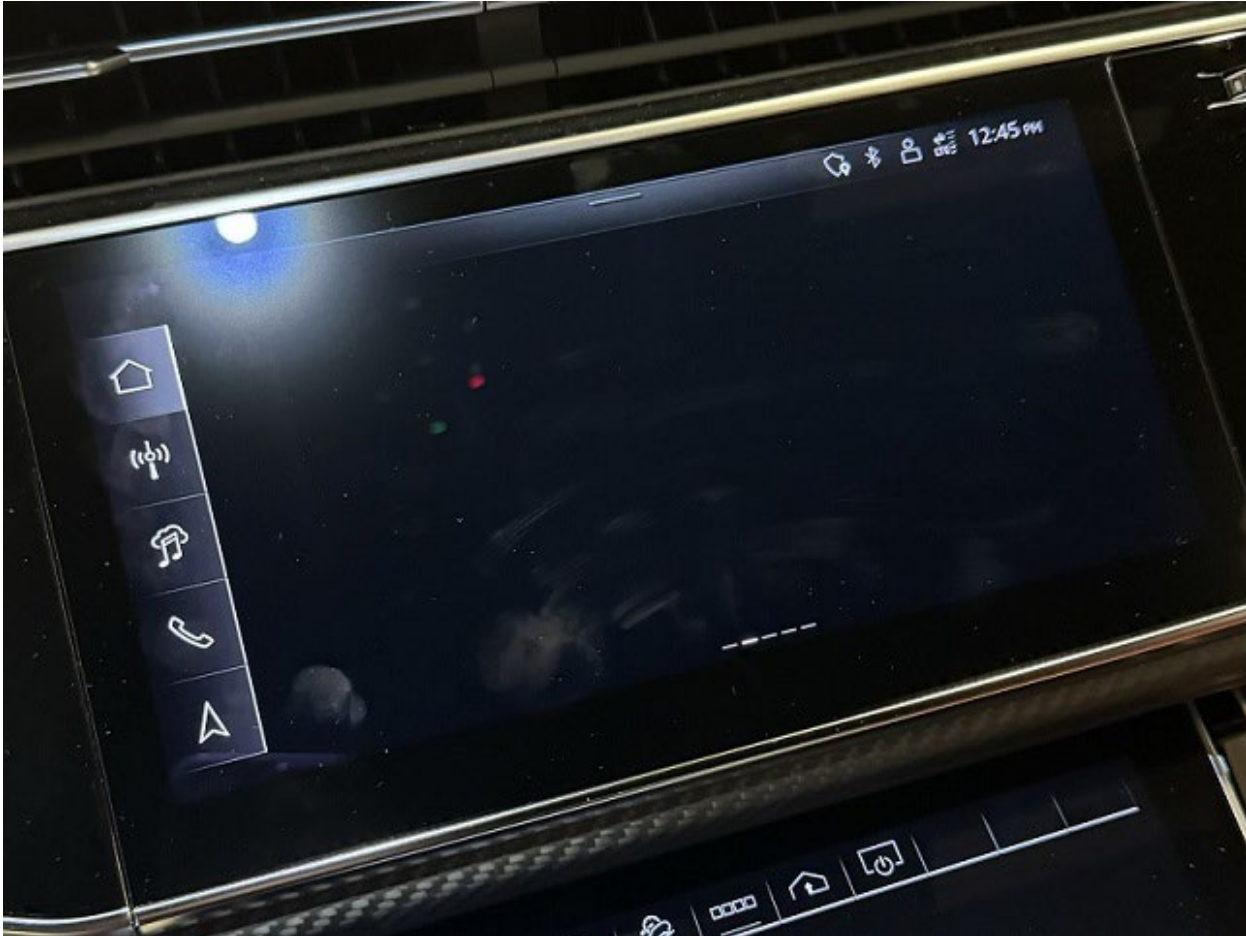
Figure 1. If icons are selected in the left menu bar when the display looks like this, the system may respond sluggishly.
