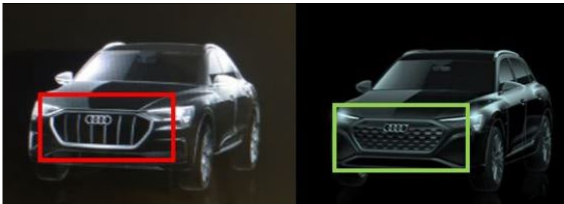
Figure 1. Radiator grille with lines (left, red rectangle) and honeycomb grill (right, green rectangle).
