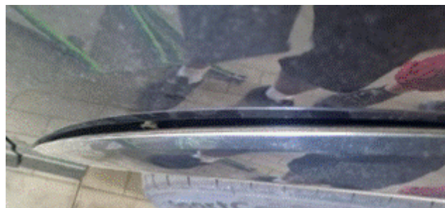
Figure 2. The front wheel arch trim with the retaining clips only partially engaged.
