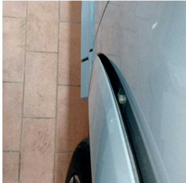
Figure 1. The front wheel arch trim is not flush to the fender surface.
