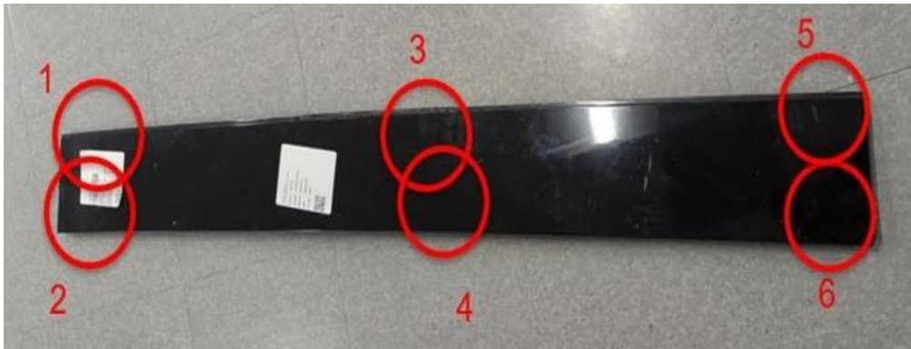
Figure 4 – Front roof applique inspection positions
