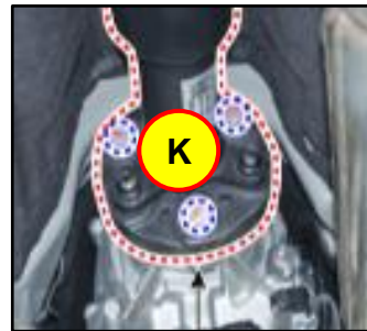
Propeller shaft to transmission/ transfer case
