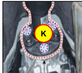
Propeller shaft to transmission/transfer case
