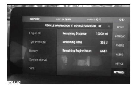
Before the head unit is flashed. Write down the service interval information.
