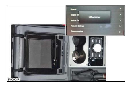
Insert the USB stick into USB-A connection in the center console storage area with Head Unit (HU) 'update' software data from software pack SW-000000773 (HU). A notification will display stating 'USB connected'
