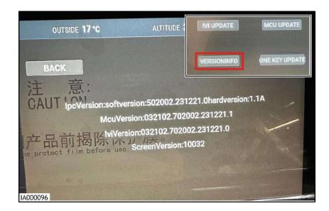
If an update fails, without functional faults, attempt the Head Unit (HU) flash of the application again. If the software application fails after 3 attempts, a Technical Support ticket should be raised. Provide the relevant information from the process step(s) to the INEOS technical support team to provide efficient support.
