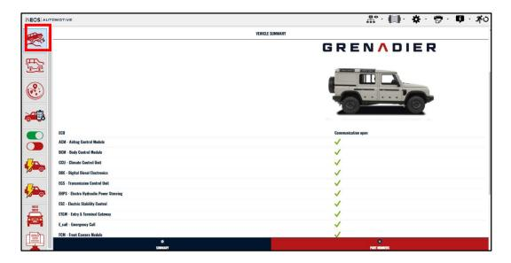
Within the 'Vehicle Summary' check all installed ECUs have an open communication displaying a green tick.
