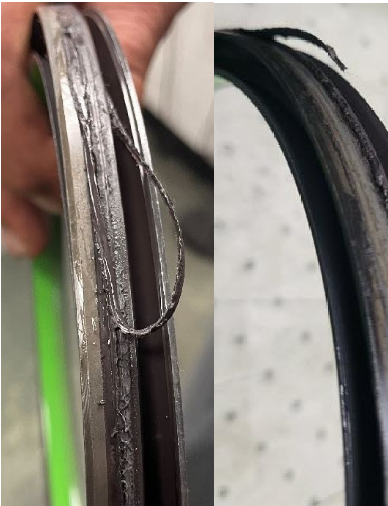
Damage to seal
