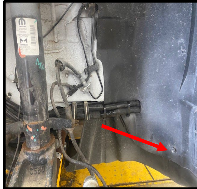
Fastener in wheel well shroud
