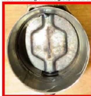
NOK mounting of valve group show this covered shaft:
