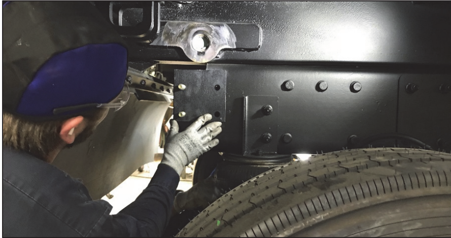
Figure 3. 4-Hole Spacer Plate Positioned Prior to Installing Lower Mounting Bracket
