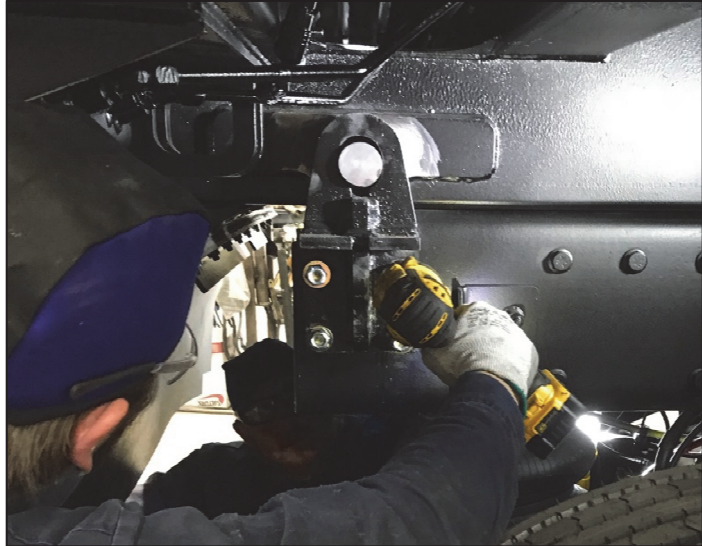
Figure 4. Position and Install Pin Mounting Weldment onto Lower Mounting Bracket, then Tack Weld Pin Mounting Weldment
