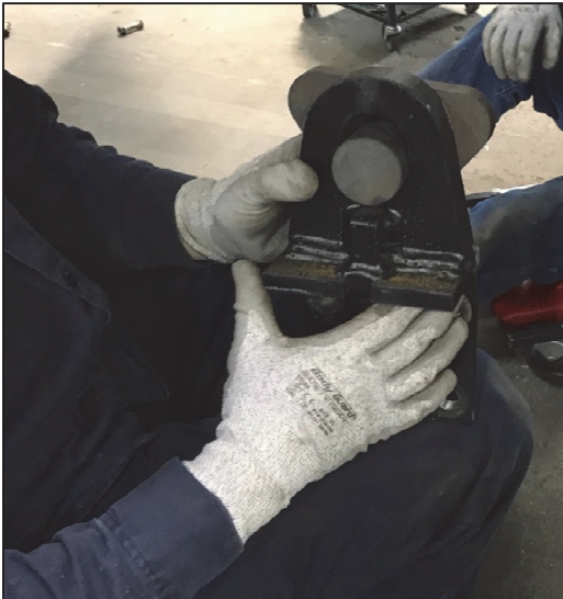
Figure 4. Position and Install Pin Mounting Weldment onto Lower Mounting Bracket, then Tack Weld Pin Mounting Weldment
