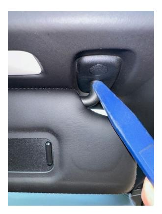
1. Unfold the passenger sun visor and check whether the shaft is fully seated.
