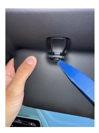
2. Remove the passenger sun visor from the end support.
