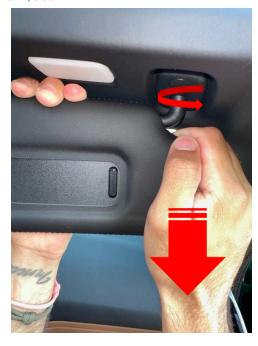
4. Pull the sun visor down with force and combine this with a swivel motion to the right and left.
