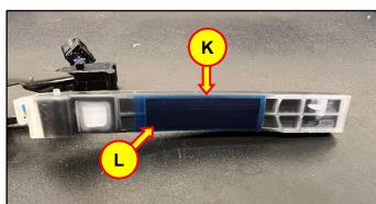
11. Firmly push down along the entire length of the double-sided tape (L) to ensure proper adhesion.
