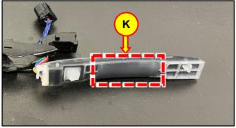
10. Apply the double-sided tape (L) to the indicated area on the touch sensor (K).
