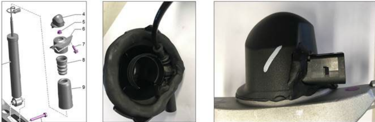
Figure 1. Example of Butyl sealing cord application and component location.
