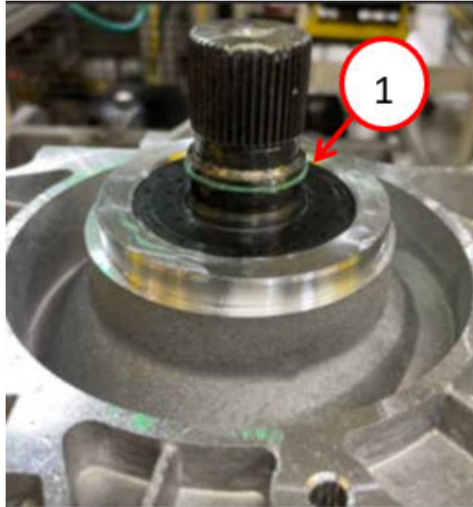
Fig. 57 Green O-Ring Installed
