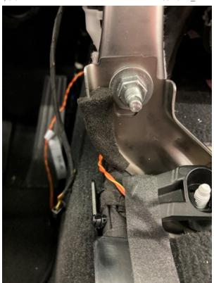
Important: The felt must be glued around the edge of the bracket!
