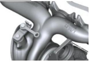
1. Inspect the wastegate lever and mechanism for corrosion.
