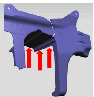
4. Do not reinstall the originally fitted cover for the steering assembly- Replace it with P/N 51 71 9 642 700.
