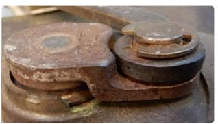
2. If the turbocharger wastegate lever is binding due to the corrosion as shown, then the complete turbocharger needs to be replaced.
