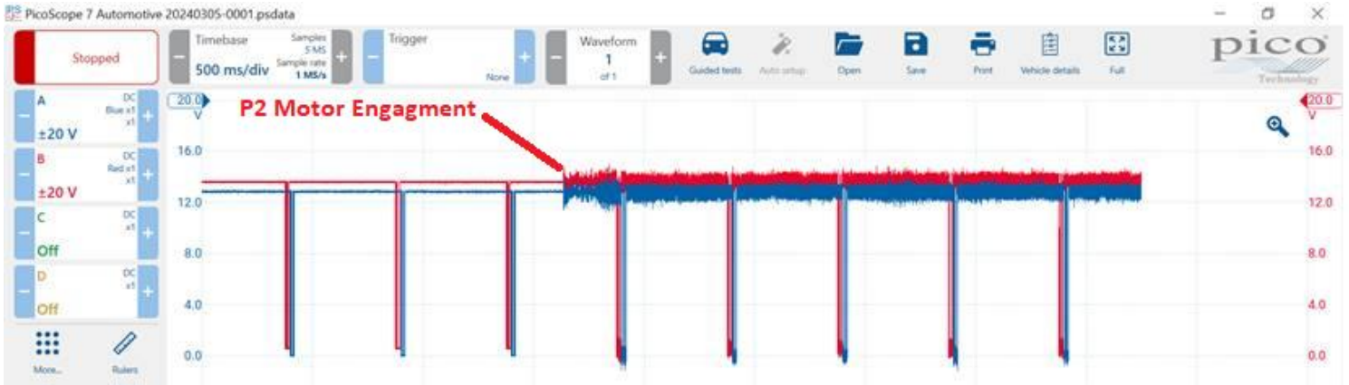
Fig. 1 :Electrical Noise on R41 and R414 Circuit After P2 Motor Engagement
