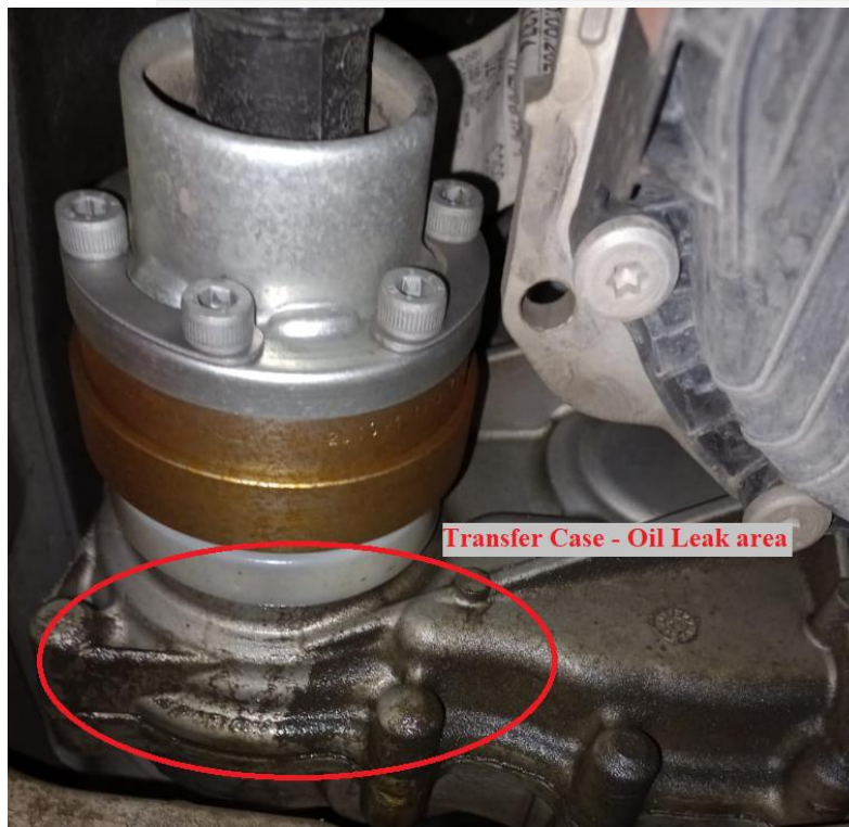
Sample of M161 – Transfer Case oil leak from the front flange area.
