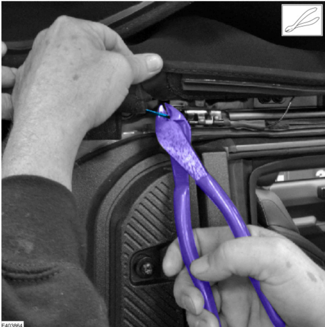
(2). Dislodge the rear spring and completely remove and discard the rear tension cable. (Figure 2) Figure 2 - Right side shown, left side similar
