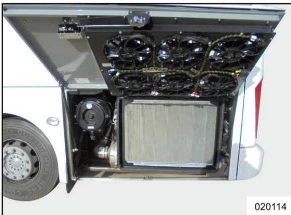
Figure 1: Radiator compartment (CX45)
