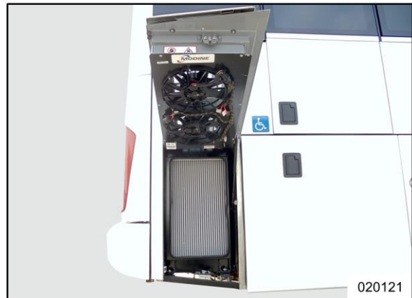
Figure 2: Charge-air cooler compartment (at RHS of vehicle) (CX45)
