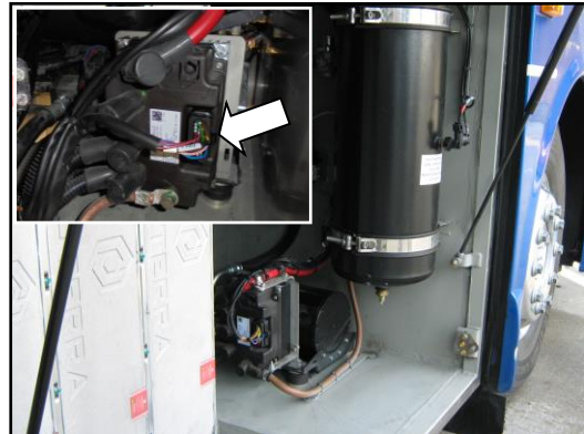
Figure 2: Location of 35-pin connector on inverter
