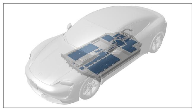
Installation position: Cell block module
