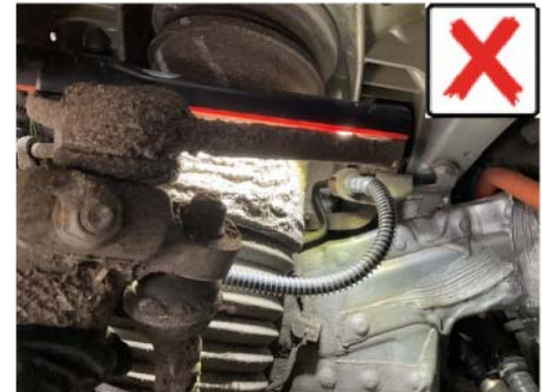
Incorrect brake hose position
