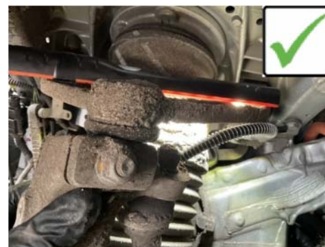
Correct brake hose position
