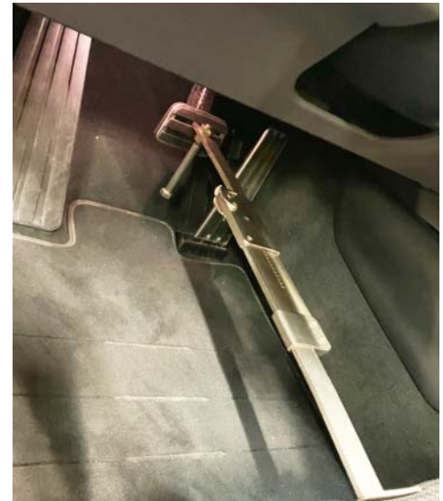
Positioning brake tensioner
