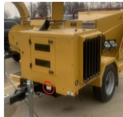
Location of Incorrect Tire Placard Decal
