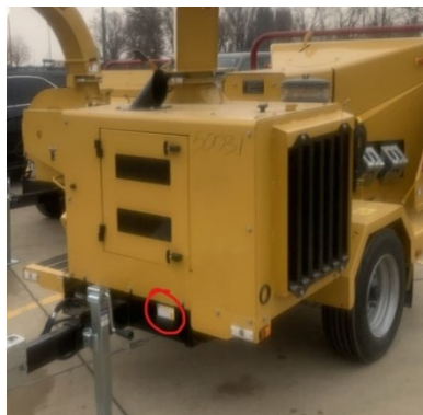
Location of Incorrect Tire Placard Decal
