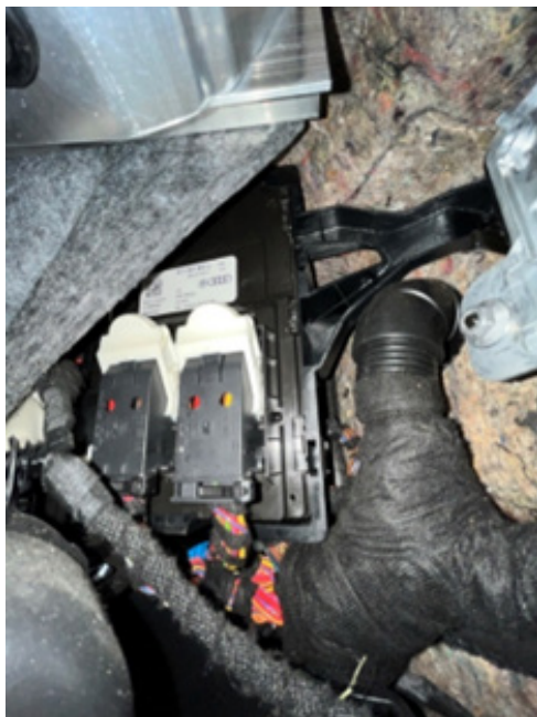
Figure 10 - Front-End Body Control Unit
