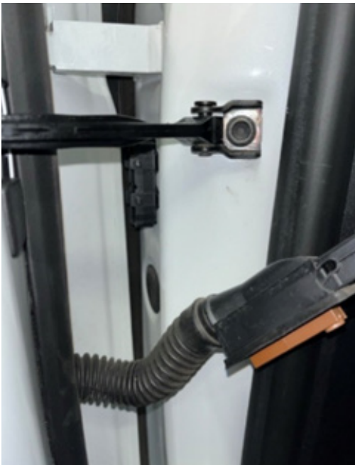
Figure 5 - Door Harness Connection Point
