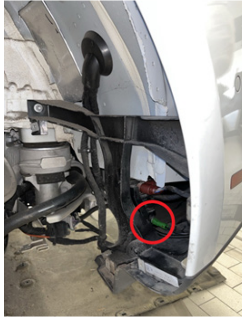
Figure 4 - Rear Camera Connection Point (Rear Driver Wheel Well)
