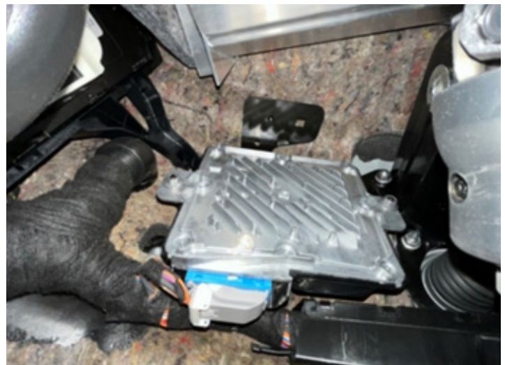
Figure 11 - Over-The-Air Function Controller
