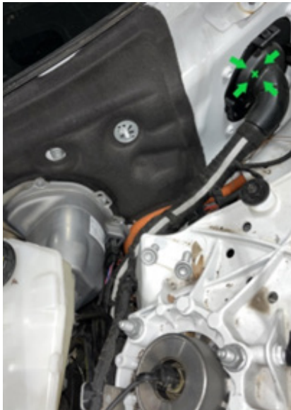
Figure 12 - Firewall Entry Point for Overlay (Under Wiper Motor)
