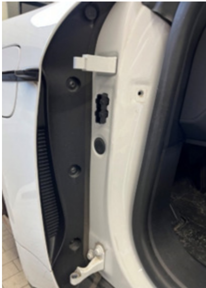
Figure 7 - Body Side Door Harness Connector
