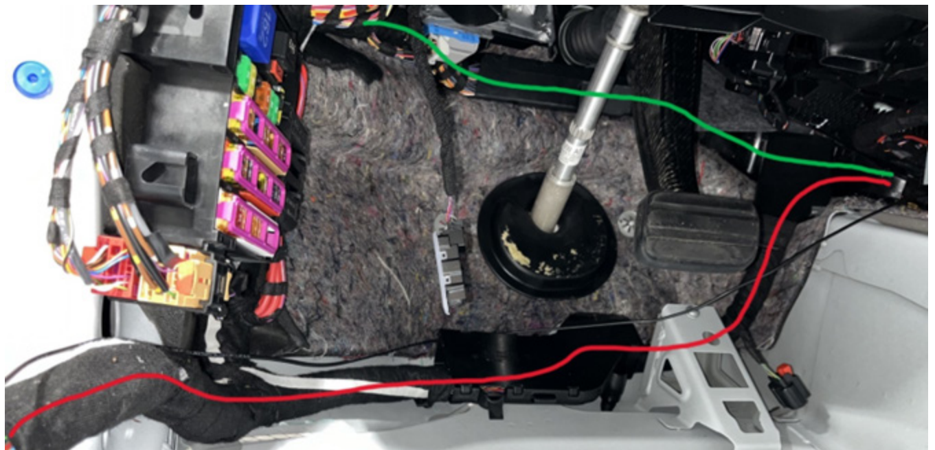
Figure 14 - Overlay Cable Pathing (Red - Rear Camera / Green - Driver Side & Front Camera)
