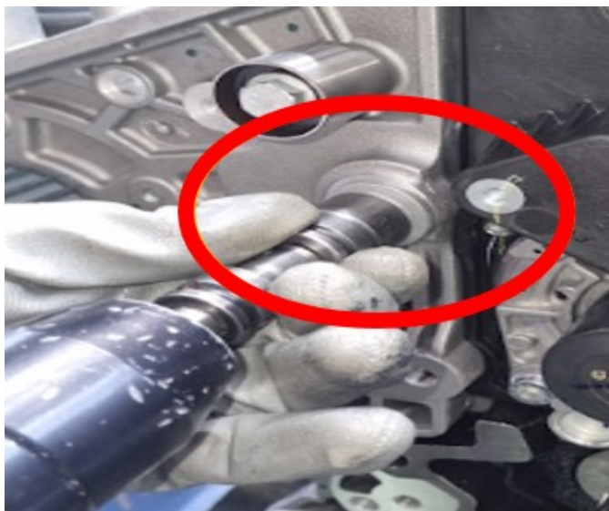
Fig. 5 Puma Bolt Tightening
