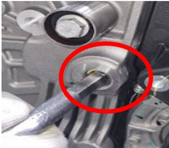
Fig. 3 Puma Bolt Loosening
