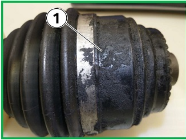
Example of dirt/contamination from outside influence (1).
