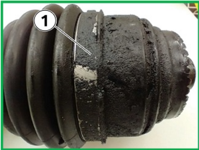
Example of dirt/contamination from outside influence (1).
