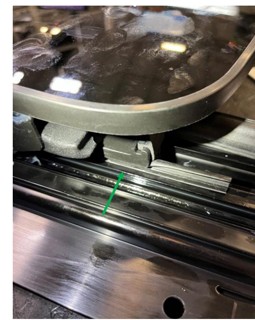
After the correction to the Dyko seal is made, it should look like the photo above. Completely behind the rear glass encapsulation.
