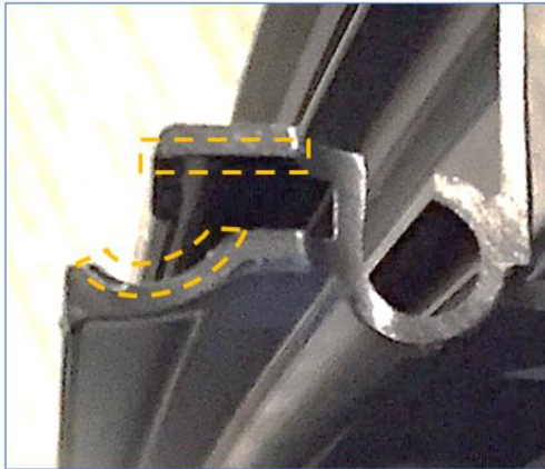
Sharp/Burr on Rollo entry at rear of guide
