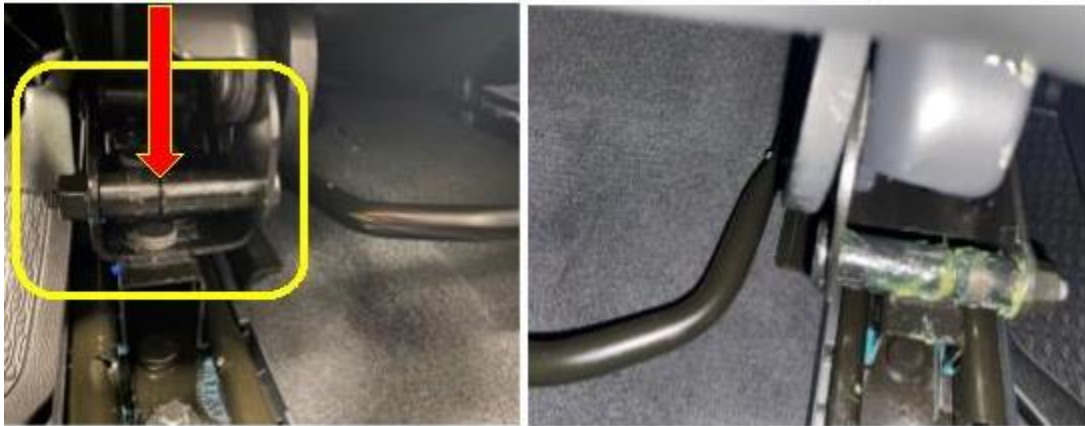
Fig 2 Application Area For Grease (Left). Grease Applied (Right).
