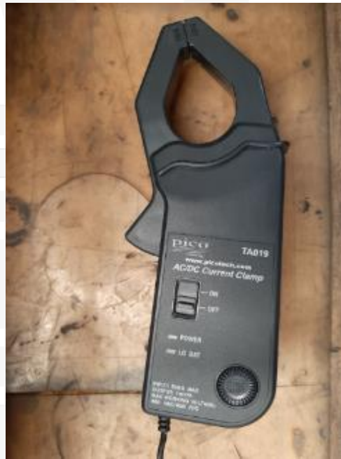
Figure 10: current clamps to be used for the measurement of current absorbed by the compressor
