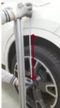
Figure 3: measuring method of the Vehicle Height at each corner.
