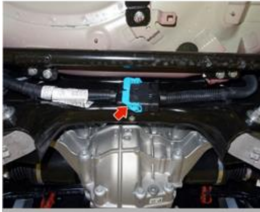
Figure 8: secondary lock (blue, indicated by the arrow) of the X090 connector..
