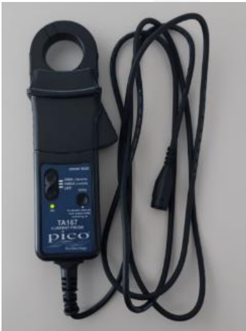
Figure 10: current clamps to be used for the measurement of current absorbed by the compressor
