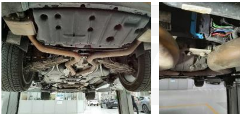
Figure 7: position of the X090 connector for the current measurement absorbed by the compressor during the actuations.
