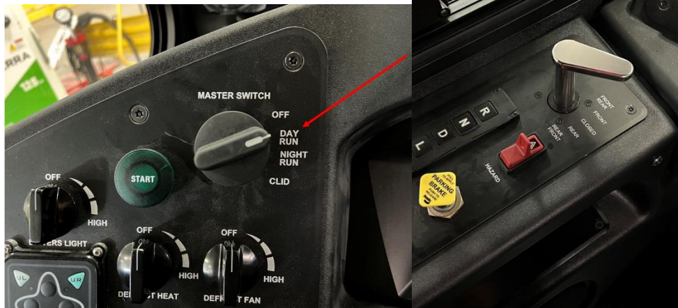
Master Switch Off, Hazards Off
