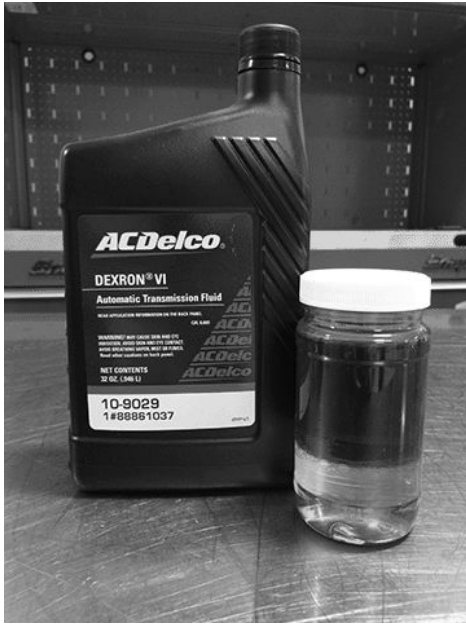
Diesel Exhaust Fluid (DEF) mixed with Transmission Fluid.
