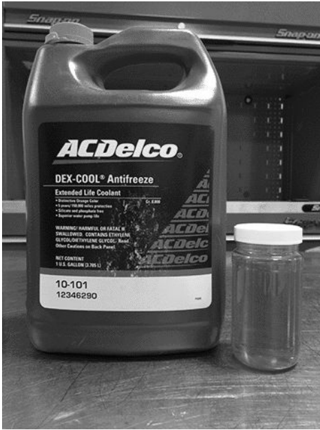
Diesel Exhaust Fluid (DEF) mixed with Dexcool.
