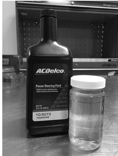
Diesel Exhaust Fluid (DEF) mixed with Power Steering Fluid.
