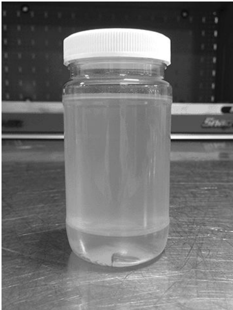
Diesel Exhaust Fluid (DEF) mixed with Diesel Fuel.
