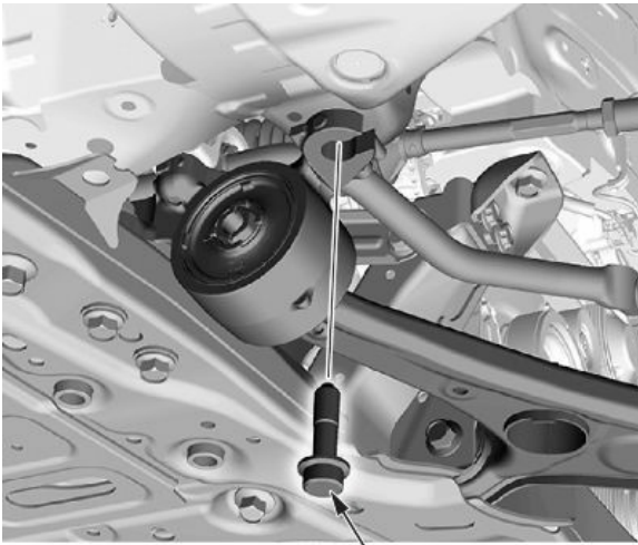
MOUNTING BOLT 69 N·m (51 lb-ft) Replace.
