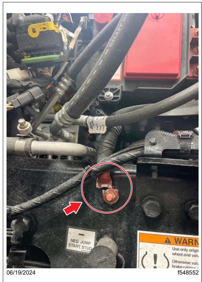
Fig. 2, Broken Ground Cable
