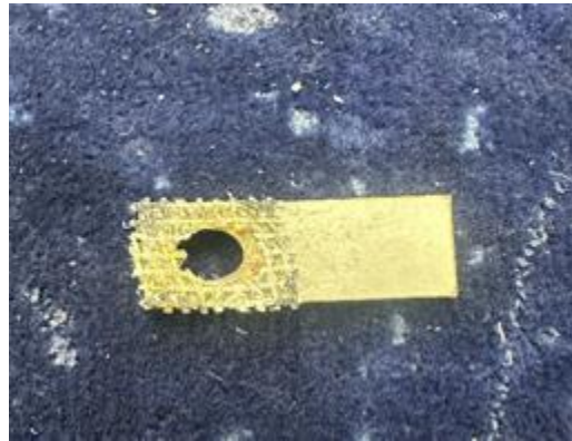
Figure 3: Apply Friction Gasket to Stopper Bracket
