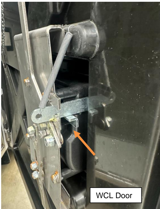
Figure 4: Adjusted Stopper Bracket with Link in Closed Position
