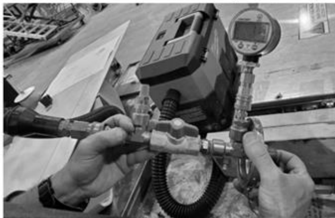
Figure 4 - Max Positive Pressure Capable with Tool (1.13 PSI)
