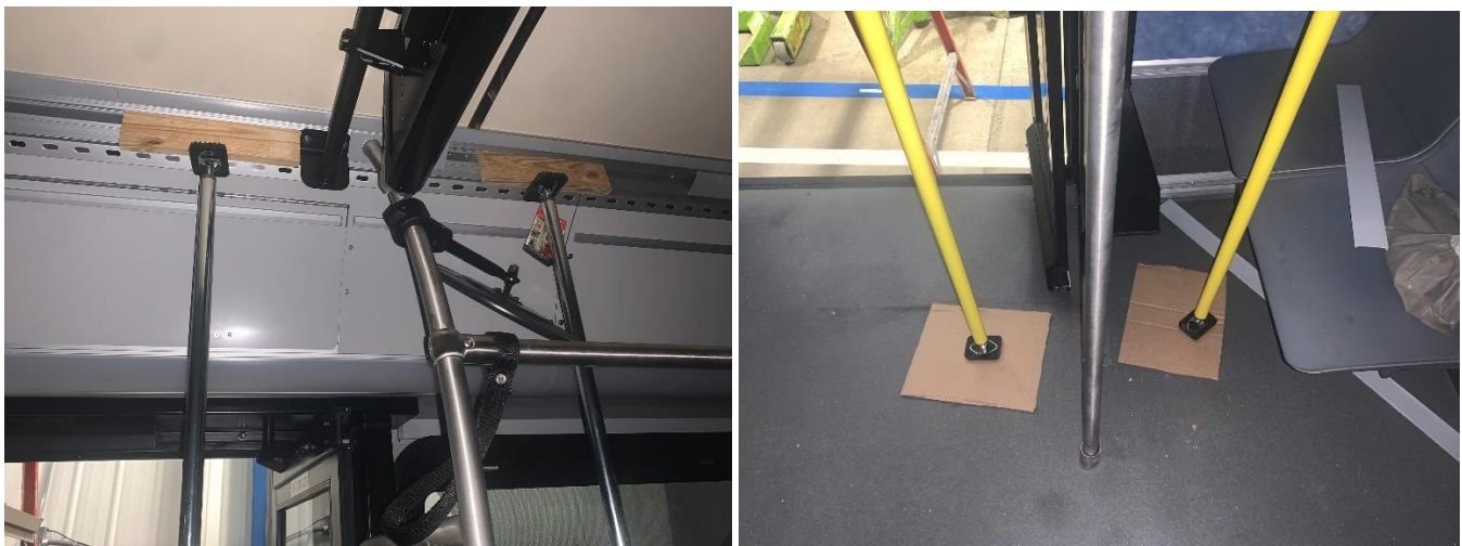
Figure 23: Wood block and support rod location reference.
