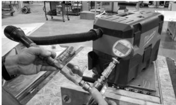
Figure 3 - Max Vacuum Pressure Capable with Tool (-0.89 PSI)
