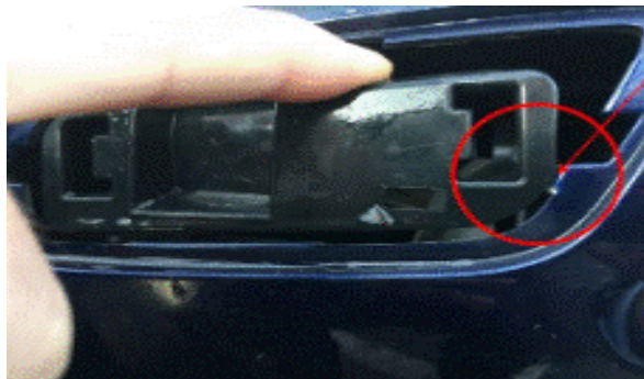
Figure 2. Interference between the headlamp washer system nozzle cover and the bumper cover.
