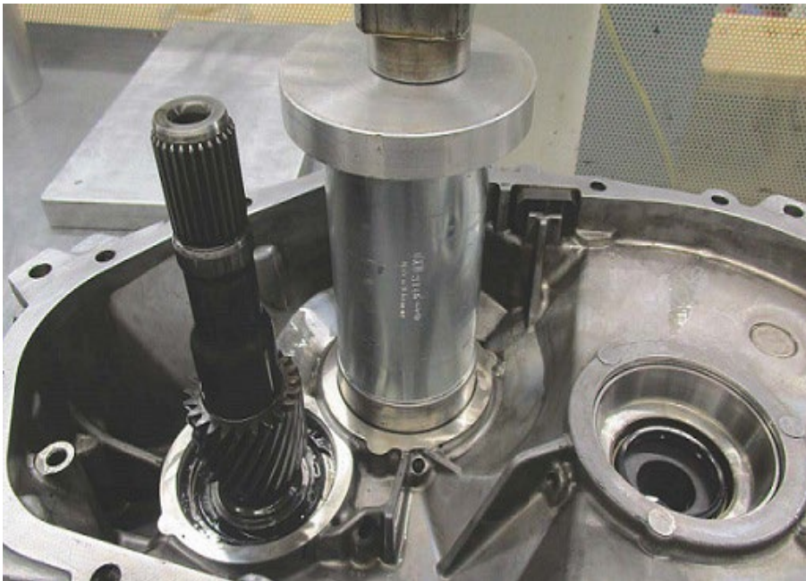
Figure 14. Pressing in new bearing for intermediate shaft with tube -3146-.
