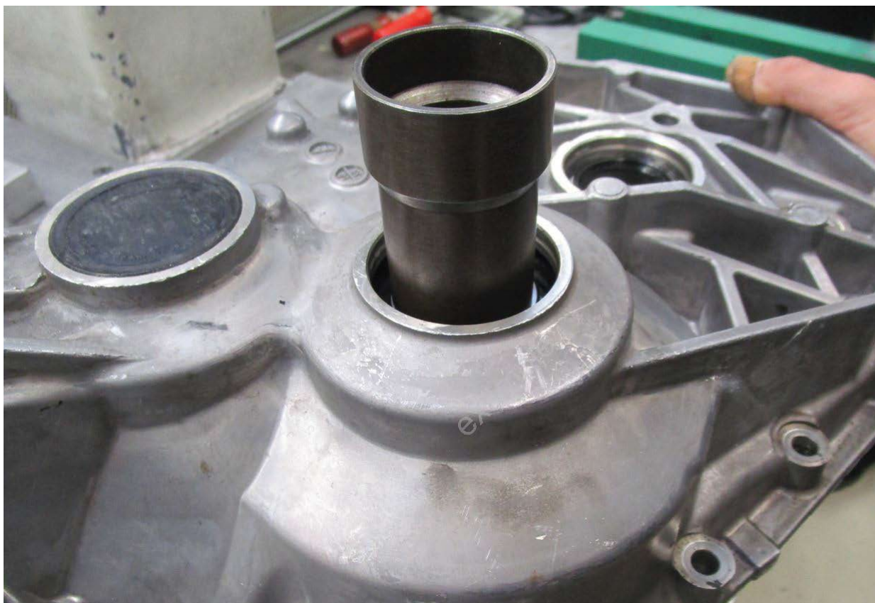
Figure 16. Supporting inner ring with thrust piece -VW454- (example).
