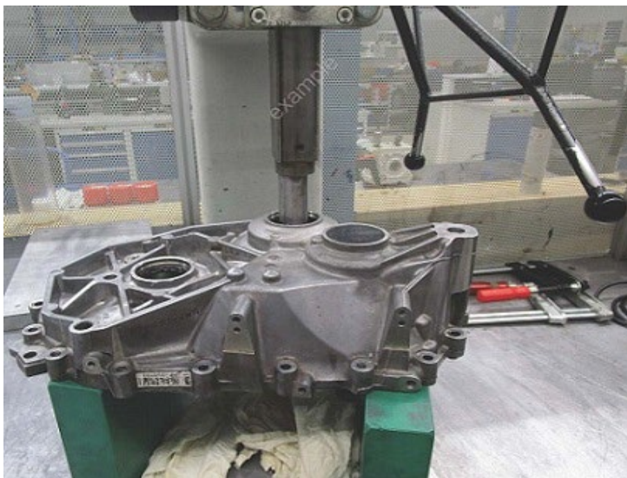
Figure 8. Pressing out intermediate shaft (example).
