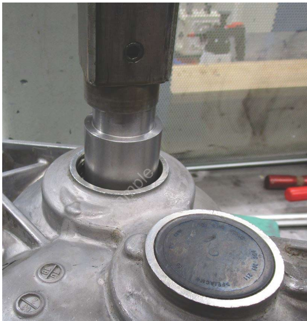
Figure 10. Pressing out bearing for intermediate shaft (example).
