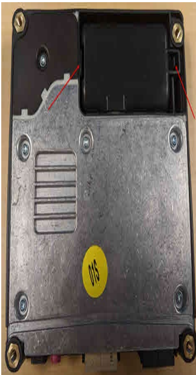
Figure 2. Backup battery compartment location.
