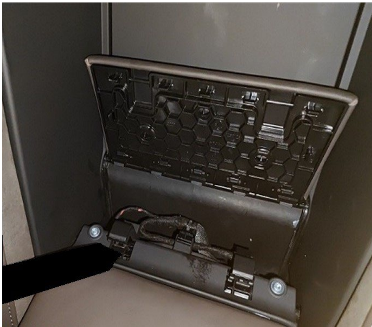
Figure 1. Broken armrest brackets
