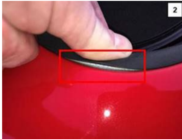
Figure 2. Checking the adhesion quality.
