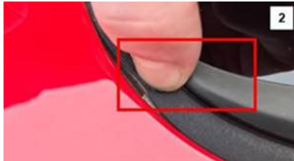
Figure 5. Clear evidence of adhesive detachment.
