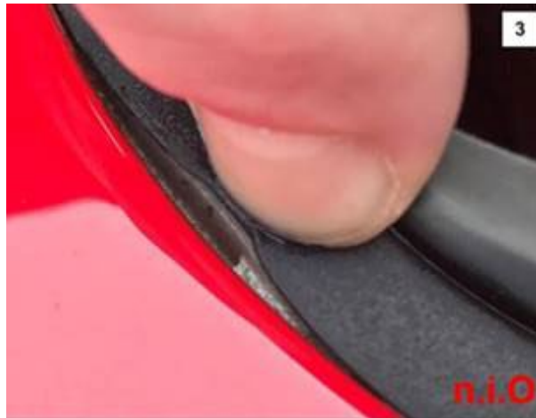
Figure 6. Seal adhesive band detachment revealed.
