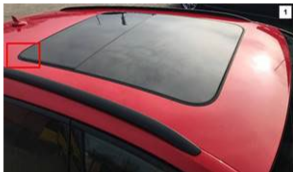
Figure 4. Begin inspection of the rear portion of the perimeter seal.
