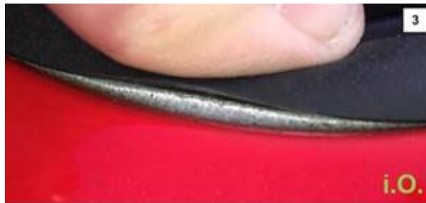
Figure 3. A properly adhered perimeter seal.
