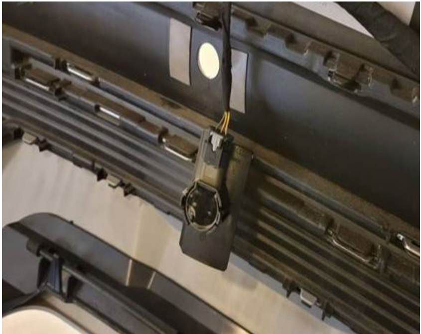
Figure 2: The parking aid mount has come loose.
