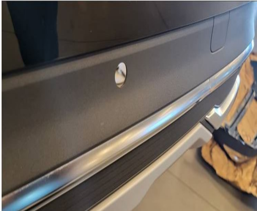
Figure 1: The parking aid mount has come loose.
