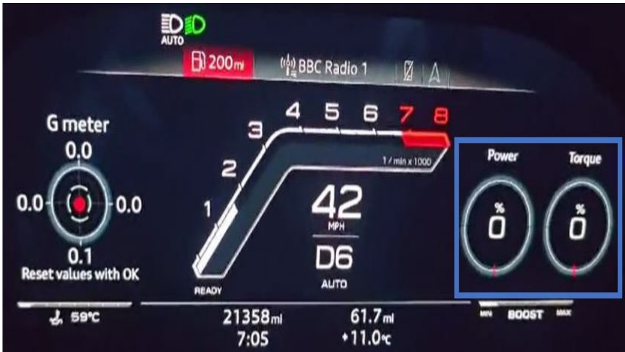
Figure 2: The power and torque displays are highlighted in the blue rectangle.
