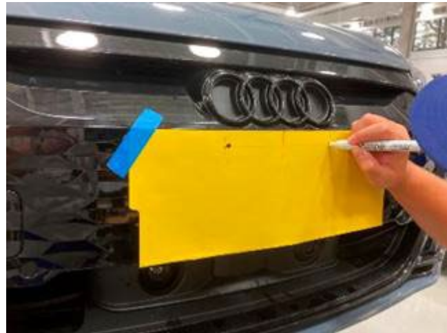
Figure 4. Screw location marking.
