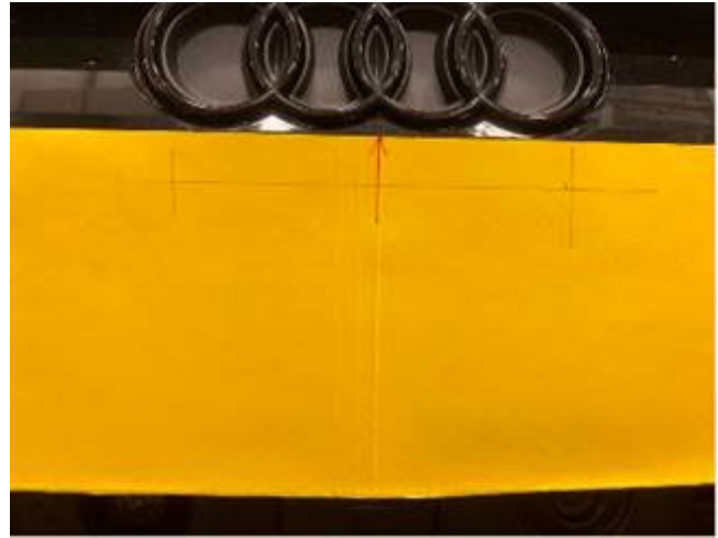
Figure 2. Front license plate mounting hole template.
