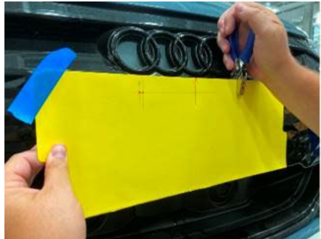
Figure 3. Hole punch through the template.
