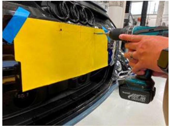
Figure 6. Drilling of the screw holes.
