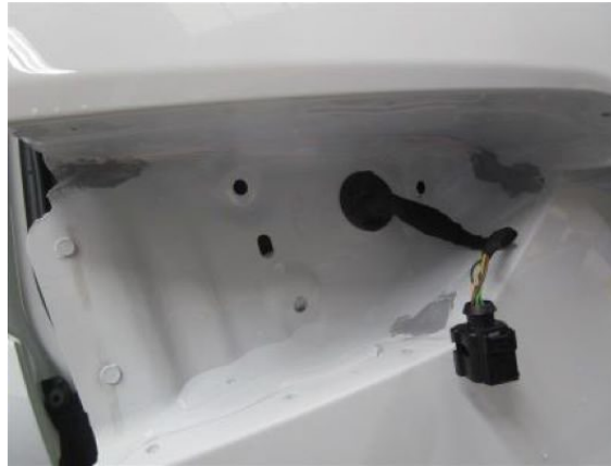
Figure 5. Concealed areas repaired with D 476KD1M2 or D 476KD1M3 sealant.
