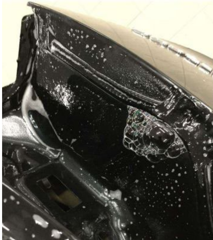
Figure 3. Bubble formation with compressed air applied internally.
