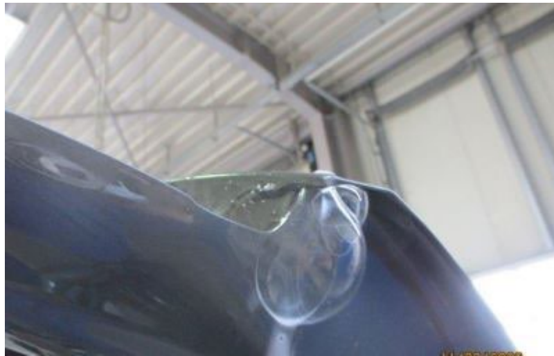
Figure 1. Bubble formation with compressed air applied internally.
