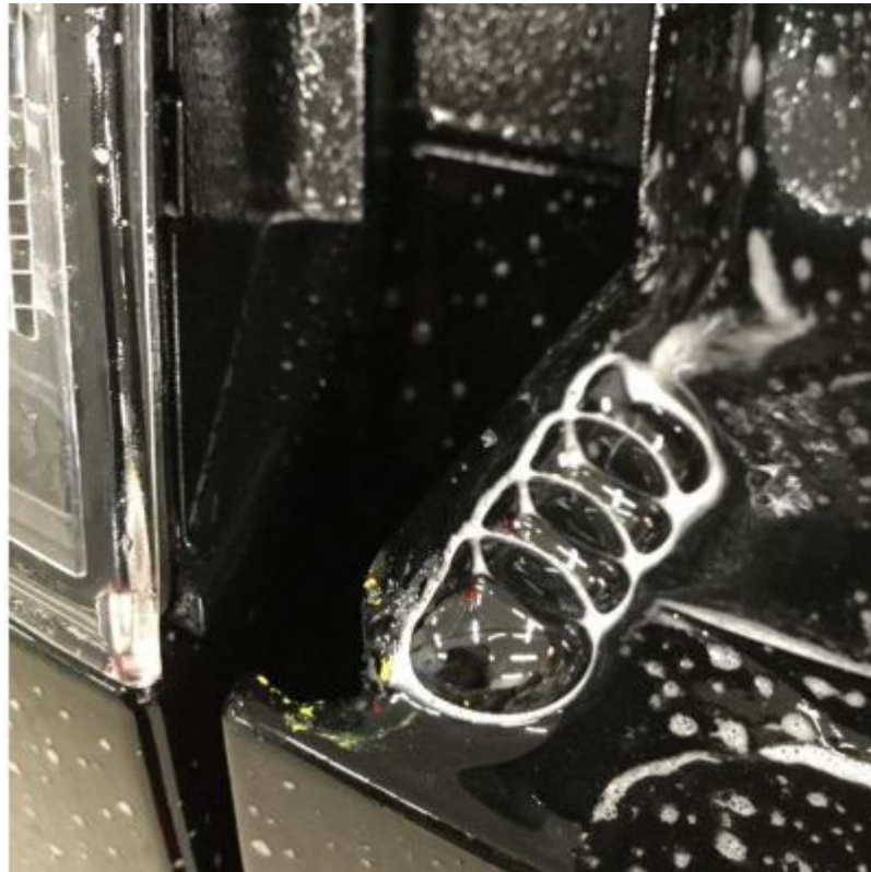
Figure 2. Bubble formation with compressed air applied internally.
