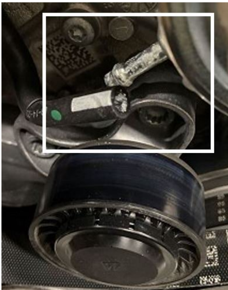
Figure 2: Dried deposits on vacuum connection.
