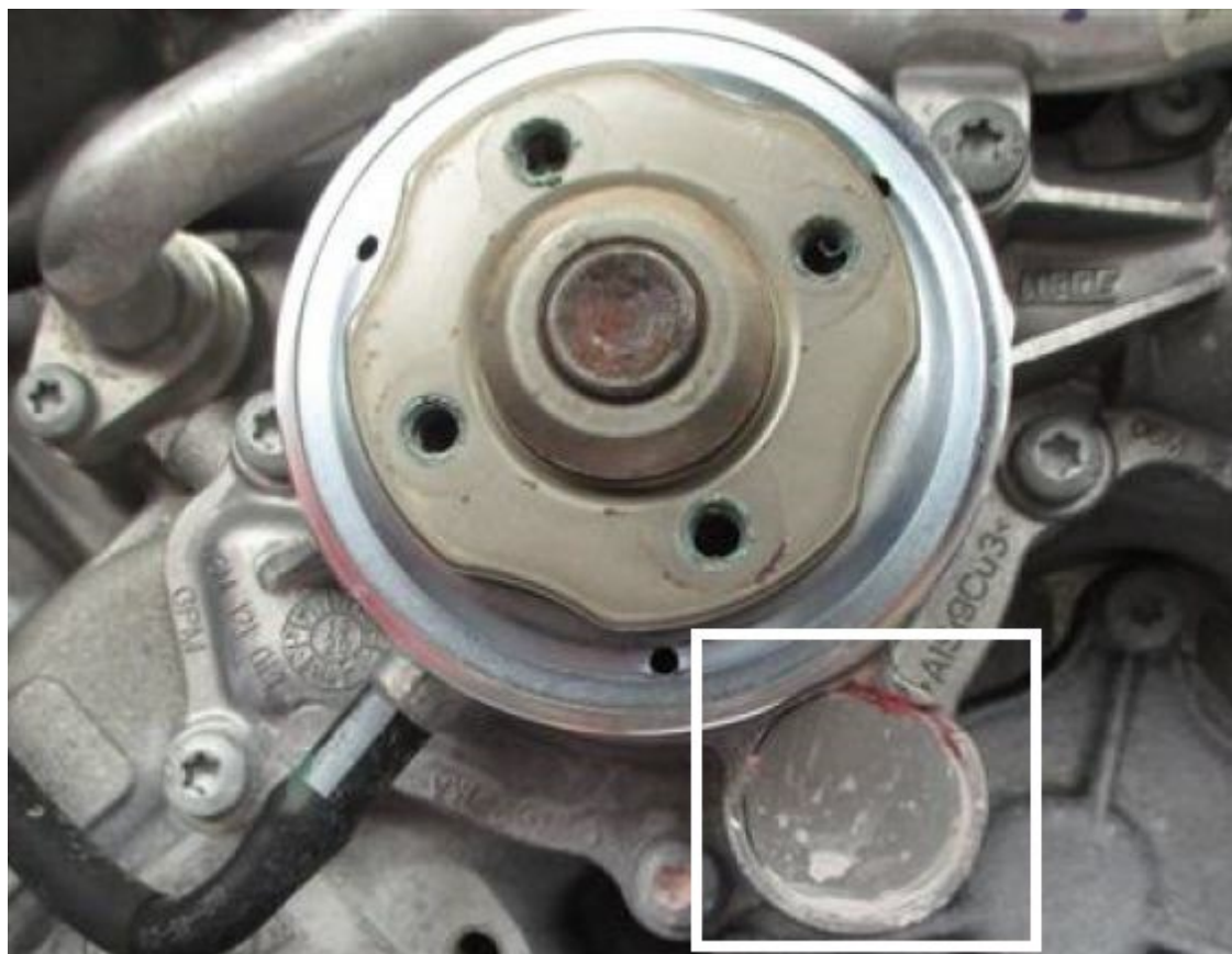
Figure 1: Traces of coolant on the drip cup.
