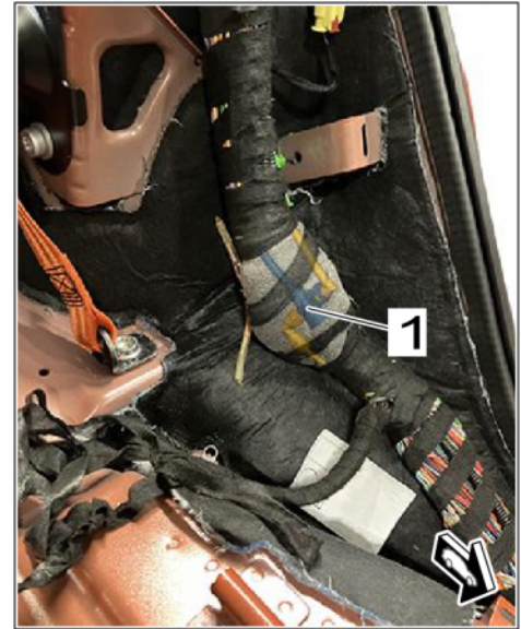
T-piece and section of corrugated tube for rear window washer system (installation position under foam shown)
