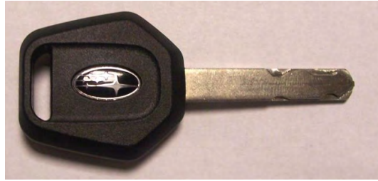
2009-2013 Forester high security laser cut key w/immobilizer
