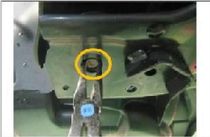
3. Once both "B" bolts are removed, clean and remove any remaining corrosion from the surface area.
