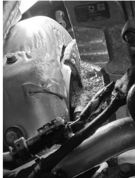
Normal turbocharger seal leakage
